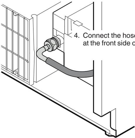
4. Connect the hose to the solenoid valve at the front side of the appliance.
