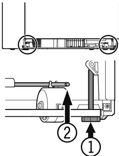
2. Adjust the height of the appliance at the rear by turning the adjusting bars ②.
