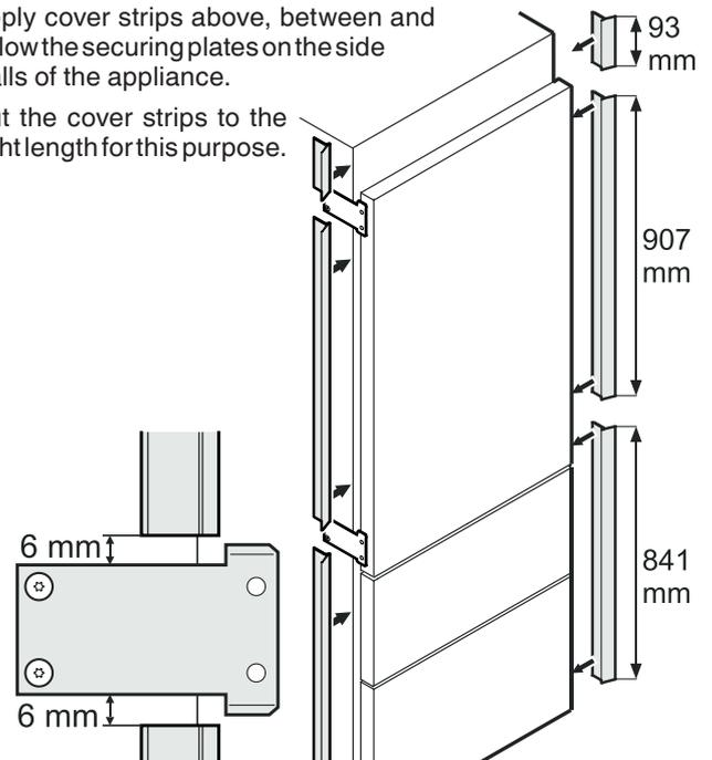
Apply the cover strips 6 mm from the securing plates.
