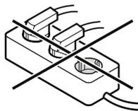
Do not use stand-alone inverters (conversion of direct current to alternating current/three-phase current) or energy-saving plugs. Risk of damage to the electronic control system!
